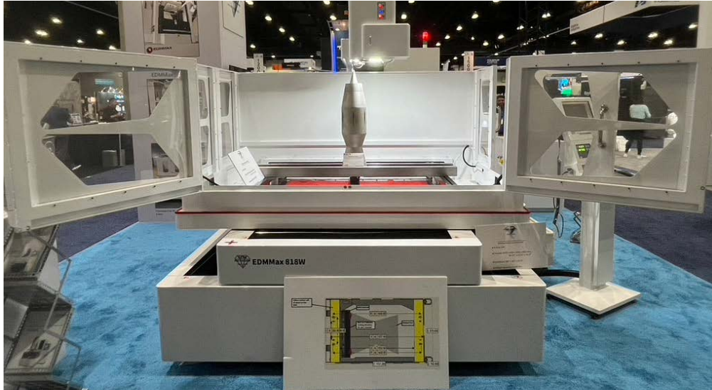
Figure 7: The EDMMax 818W fast wire electrical discharge machining (EDM) system from EDM Network Inc.
