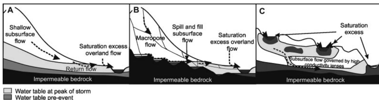
Figure 1. Principle 1: Delineate hydrological systems by considering the dominant processes and pathways of water: (A) variable source area hydrology where surface topography controls hydrological flows, (B) variable source area hydrology where bedrock topography controls hydrological flows, and (C) nonvariable source area hydrology in sub-humid, flat landscapes where surficial geology controls hydrological flows (from Creed and Sass, 2011)
